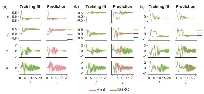
FIG. 17. NGRC models can fail to reproduce the correct transient dynamics even when the attractor is correctly predicted. Counterpart to Fig. 8, showing examples of training initial conditions for which the NGRC predicted trajectory (green, right columns) goes to the correct attractor, but the transient dynamics differs markedly from the ground truth (pink). All hyperparameters are the same as in Fig. 8.
