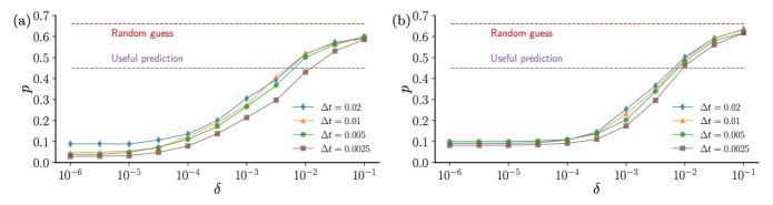
FIG. 21. NGRC basin prediction accuracy when using the exact nonlinearity but with small uncertainties. Same as Fig. 7, but with the height of the pendulum set to (a) h = 0.3 and (b) h = 0.4.
