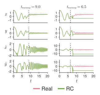
FIG. 14. Sensitivity of standard RC performance to warm-up time. Counterpart to Fig. 3 with the initial condition  $(x_0, y_0) = (1.75, 1.6)$ . The respective warm-up times indicated by the dashed lines are the same as in Fig. 13.
