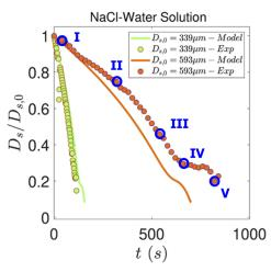
FIG. 3. Instantaneous droplet images taken by a CCD camera (top left panel) and dark field micrograph of the final salt precipitate (top right panel). Comparison of experiments and simulations in the bottom left and right panels. Evolution of the normalized droplet diameter as a function of time for pure water (left panel) and the salt water solution droplet with 1% NaCl (right panel).
