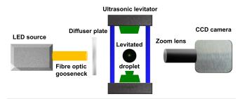
**FIG. 1.** Experimental setup showing the acoustic levitation of a droplet illuminated by a cold LED source. A diffuser plate is used for uniform imaging of the droplet. A CCD camera fitted with the zoom lens assembly is used for illumination. The schematic is not to scale.
